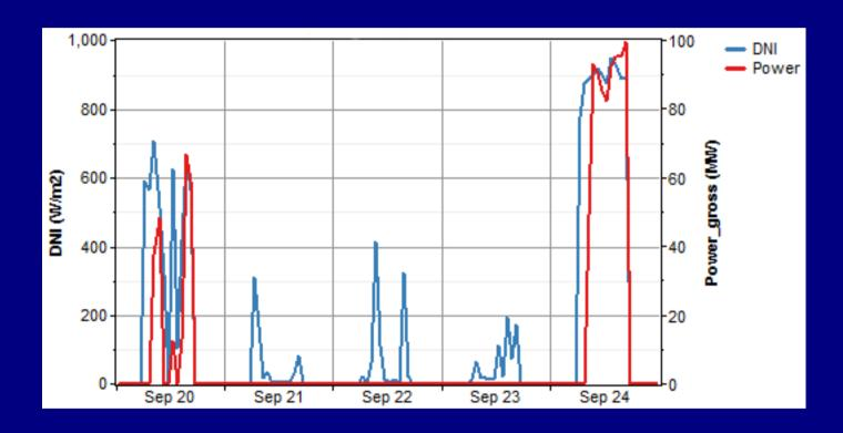
Simulated 100MW trough plant in Cobar, NSW, September 2009
