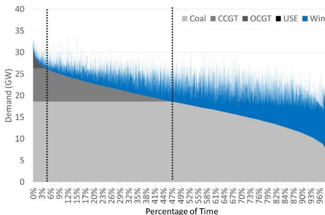
With these cost assumptions, as the level of wind penetration increases to 25GW, 6.8 GW of coal-fired generation is displaced. This is partially replaced with an increase of 4GW of CCGT and 300MW of OCGT plant, as illustrated in Figure V.5. The least cost optimized capacities are listed in Table III. Due to the relatively high cost of gas, coal-fired generation is favored (compared to the previous scenarios depicted in Table II), despite the moderate carbon price.
