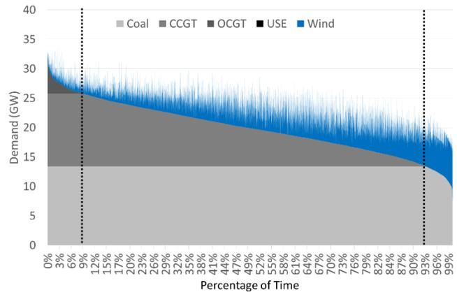
Figure IV.3 - Least cost optimized results for High Wind Scenario (25GW wind installed)
