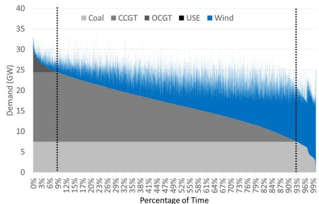
Note that anomalies in the right hand side of the wind generation curve are present in the original wind data collected from operating wind farms, and are thought to be due to curtailment during low demand periods.
