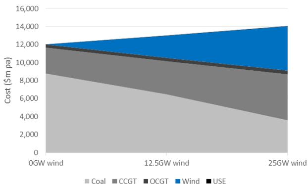
Wind generation acts to significantly reduce the balance of system costs (the total system costs, minus the costs related to the wind generation itself). Adding 12.5GW of wind reduces
