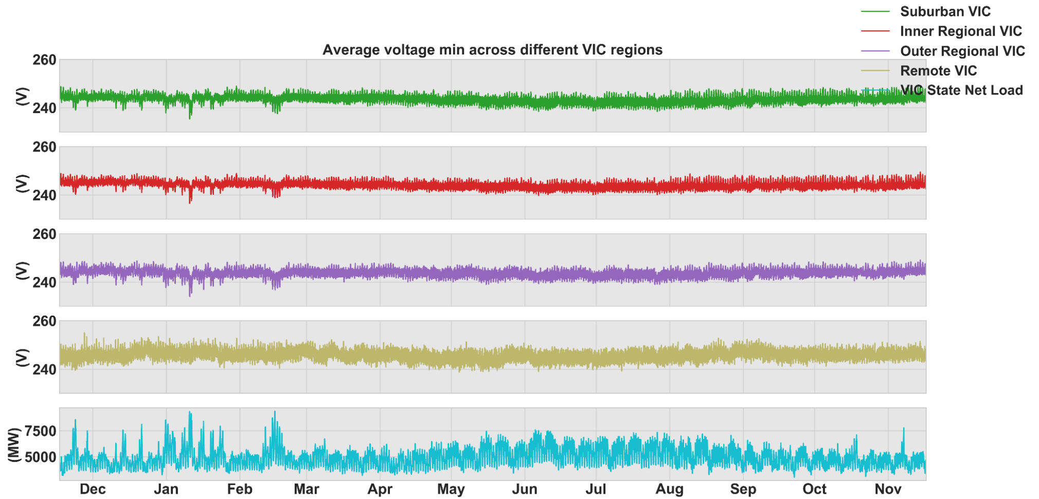
Figure 61 Average voltage minimum across different regions of Victoria and the net state load
