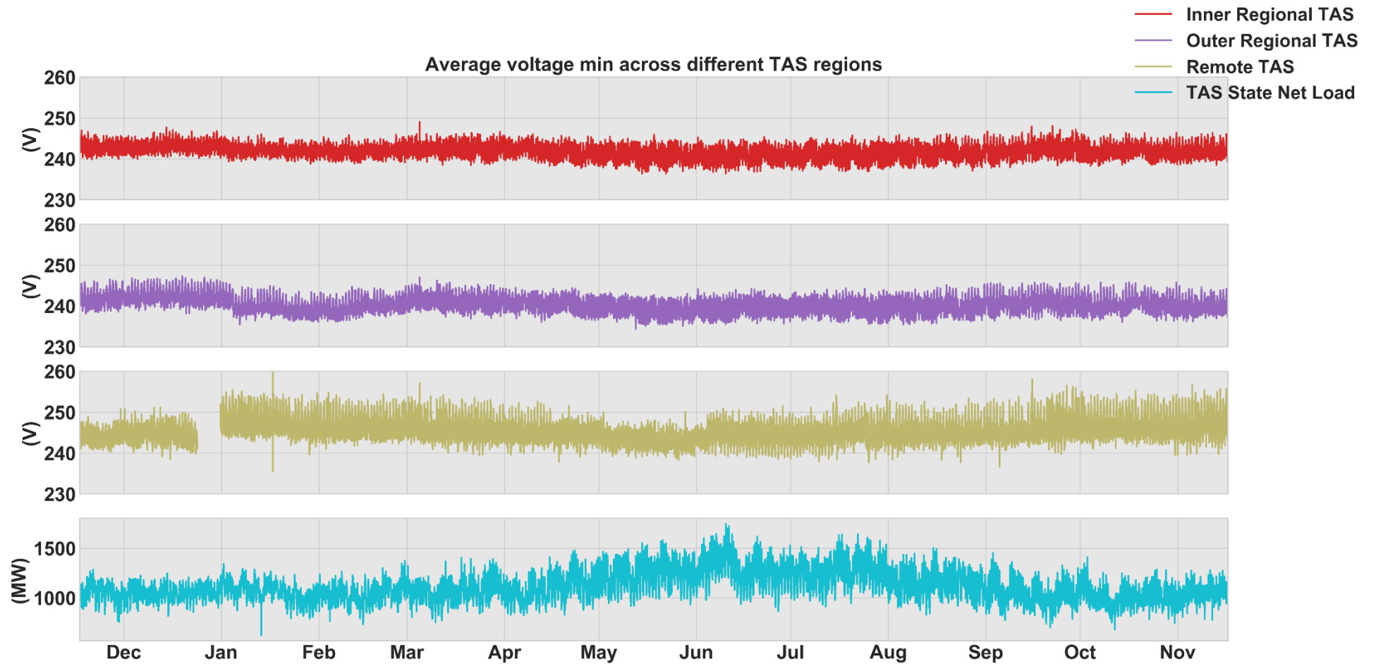
Figure 90 Average voltage minimum across different regions of Tasmania and the net state load
