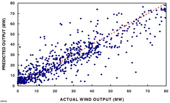
Figure 2. Two-hour predictions of power output from the Lake Benton wind farm compared to actual power output, with the red line corresponding to a perfect prediction (Hirst, 2001)
