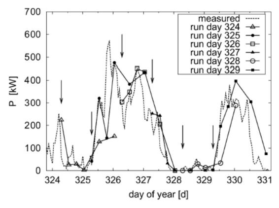
Figure 3. Comparison of measured and predicted output of a wind turbine (Focken et al, 2002). The downward pointing arrows show the first (6 hour) forecast in each set of 6, 12, 18, 24, 36 and 48-hour forecasts. The 6 and 12-hour forecasts are always accurate in this example.
