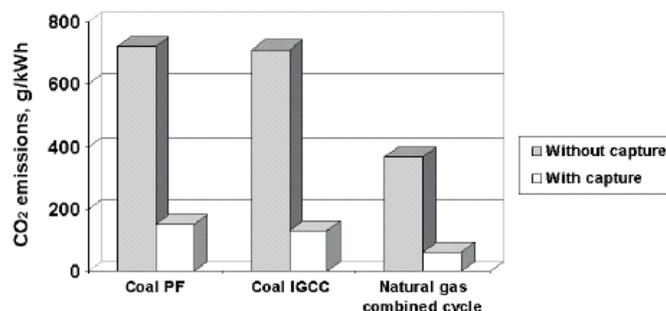
**Figure 2:** CO<sub>2</sub> emissions from different fossil fuel generation options with, and without, CO<sub>2</sub> capture (taken from IEA, 2001).
