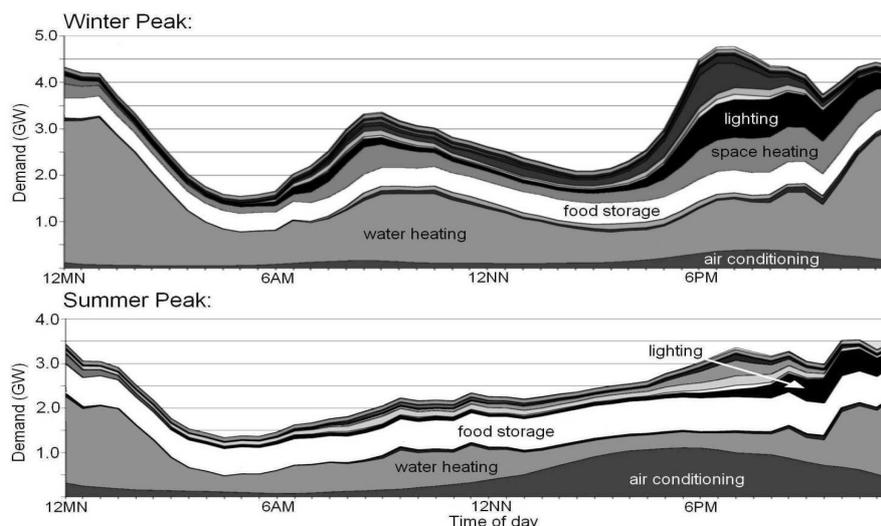
Figure 1: Total peak electricity demand of the residential sector in New South Wales, Australia, broken down by application, in June 2002 and January 2003. These are edited versions of the original figures in [Consultant Pty Limited, 2004].
