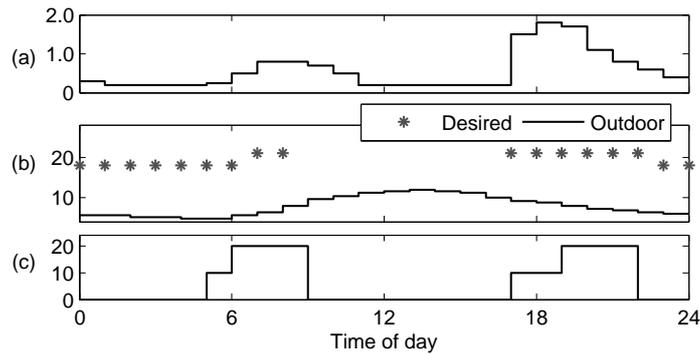
Figure 3: Hourly demand for the energy services: (a) Must-run service power consumption, in kW; (b) Heating service: required hourly temperature, in °C, the outdoor temperature is also shown; (c) Hot water service: hot water consumption, in liters.
