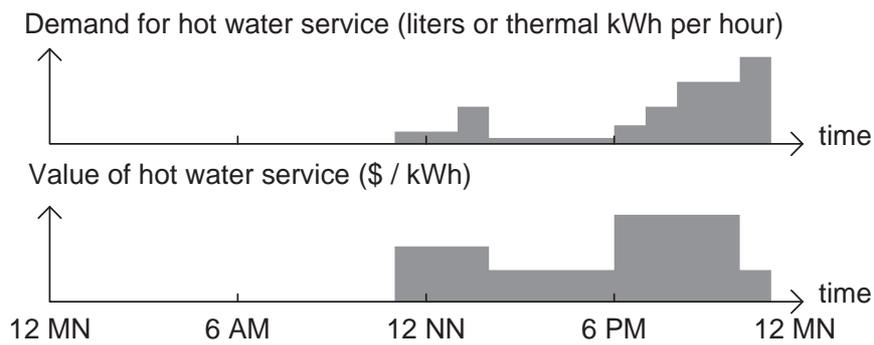
Figure 2: An example of how to use the proposed energy service model to describe the demand for and benefit of hot water service in a restaurant.
