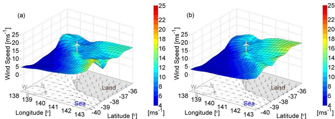
**Figure 1: (a) raw and (b) standardised wind speed fields for an ECMWF forecast with projection time 15 hours ahead. Each plot (a) and (b) shows the wind speed fields in a 3D plot with the wind direction field shown on a 2D plot beneath it. The wind turbine symbol indicates the modelled location of the wind farm. Note how the standardised field has generally lower wind speeds over the ocean and higher over land compared with the raw field.**
