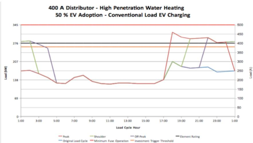
Fig. 2: High Penetration Water Heating - Peak, Shoulder and Off-Peak Charging Regime – 50 % EV adoption 160 km scenario
