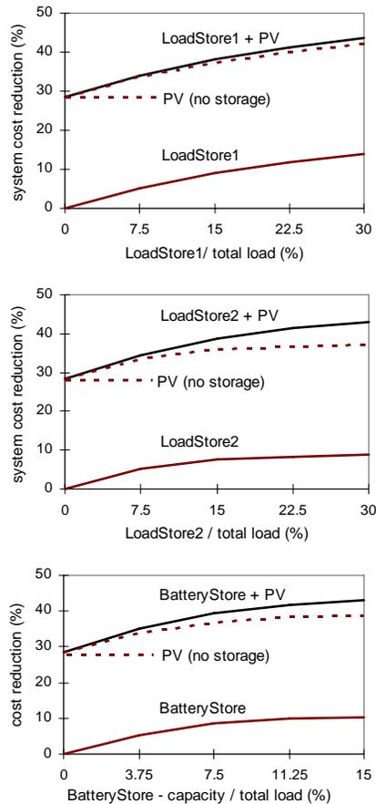
**Figure 8. Reduction in system operating costs for increasing storage penetrations without PV, and with 70% PV penetration. The dotted line represents what cost reductions might be expected from PV and storage if no synergies existed.**
