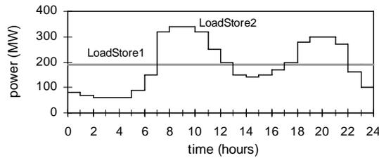
**Figure 5. Daily demand profiles for the two distributed loads with inherent energy storage.**
