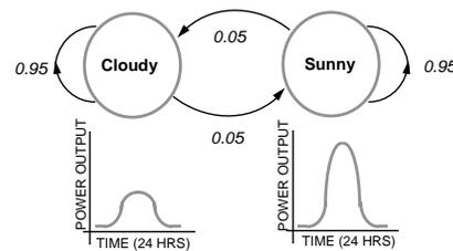
**Figure 4. Markov-chain of PV output for Monte-Carlo simulations of power system operation.**
