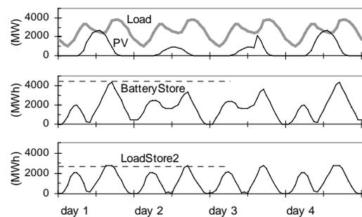
**Figure 7. Simulated operation of power system over four days with optimal storage behaviour.**
