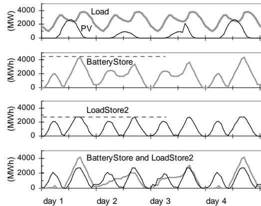
**Figure 9. Simulated operation of power system as for Figure 7, but now including optimal storage operation when both storages are present.**
