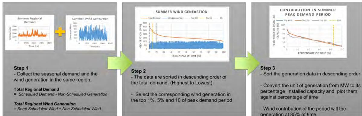
**Figure 1: Flowchart outlining the AEMO Approach to calculating wind capacity value in the NEM**
