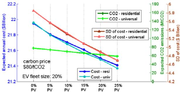
Figure 11. Expected costs, SDs and CO<sub>2</sub> emissions of the lowest cost generation portfolios for different PV penetrations in the case of \$80/tCO<sub>2</sub> and 20% EV. Note that the CO<sub>2</sub> and SD of cost curves are largely overlapping for both infrastructure cases.
