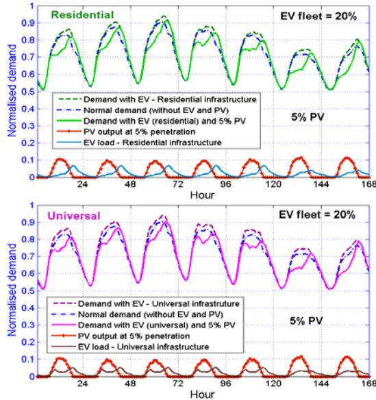
Figure 1. Weekly demand, PV output and EV load during a typical summer week for residential and universal charging infrastructure cases.
