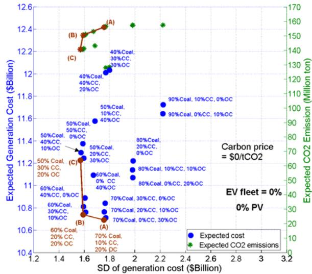
Figure 5. Expected annual system costs, cost uncertainty and CO<sub>2</sub> emissions of generation portfolios for the case without EV, PV or a carbon price. The expected costs are represented by the circles and the CO<sub>2</sub> emissions of the corresponding portfolios are represented by the asterisks in the same vertical line.
