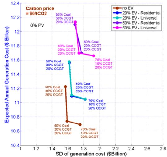
Figure 6. Cost-risk efficient frontiers for different EV fleet sizes in the case without a carbon price and PV generation.
