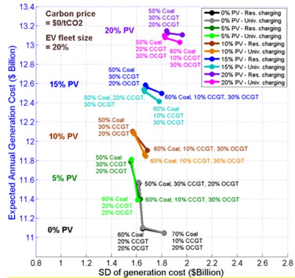
Figure 7. Cost-risk efficient frontiers for different PV penetrations
