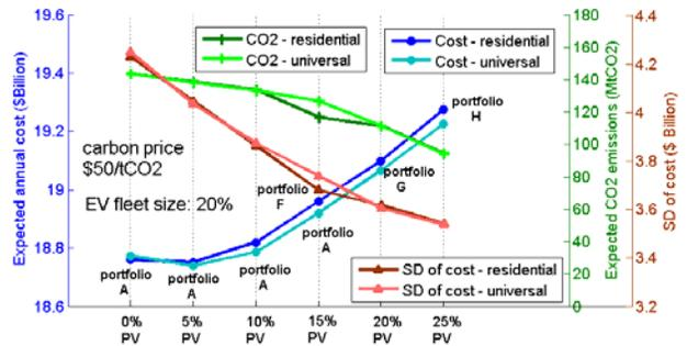
Figure 10. Expected costs, SDs and CO<sub>2</sub> emissions of the lowest cost generation portfolios for different PV penetrations in the case of \$50/tCO<sub>2</sub> and 20% EV.
