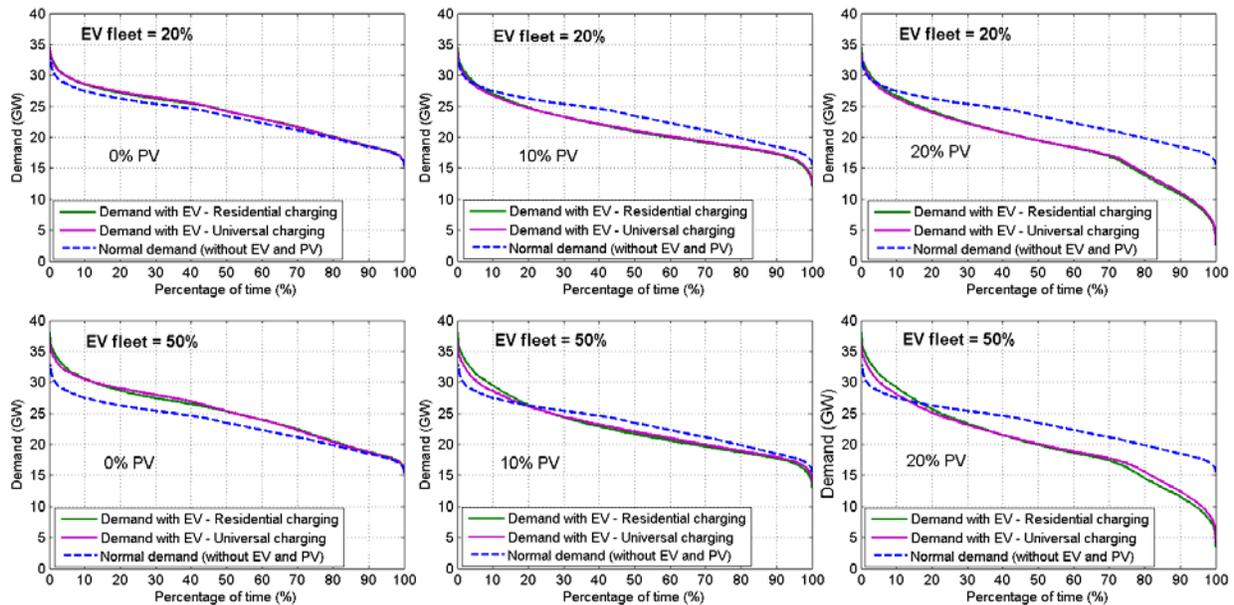
Figure 2. LDCs and RLDCs for different EV fleet sizes and PV penetrations for different charging infrastructure scenarios.
