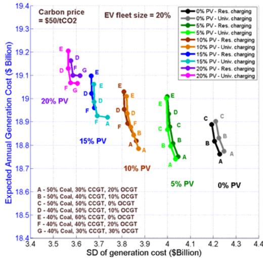
Figure 8. Cost-risk EF showing optimal generation portfolios for different PV penetrations in the case of \$50/tCO<sub>2</sub> and 50% EV.
