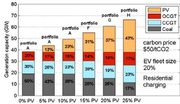
Figure 9. Installed capacity of each technology of the lowest cost portfolios for different PV penetrations in the case of \$50/tCO<sub>2</sub> and 20% EV.
