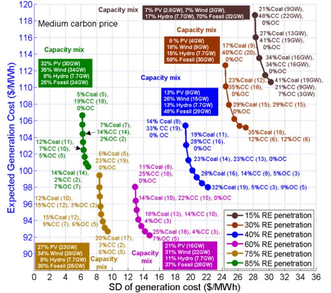
Fig. 1. Efficient frontiers containing optimal generation portfolios for different renewable penetrations in 2030. The capacity of fossil-fuel technologies in each portfolio is shown in GW (in brackets) and percentage share. The coloured boxes show the share of each technology by capacity installed.
