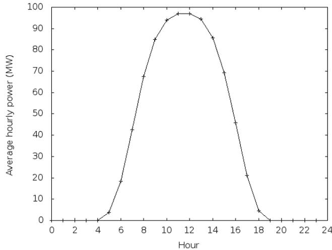
Figure 1: Typical power curve for a fixed 100 MW PV system in clear sky conditions
