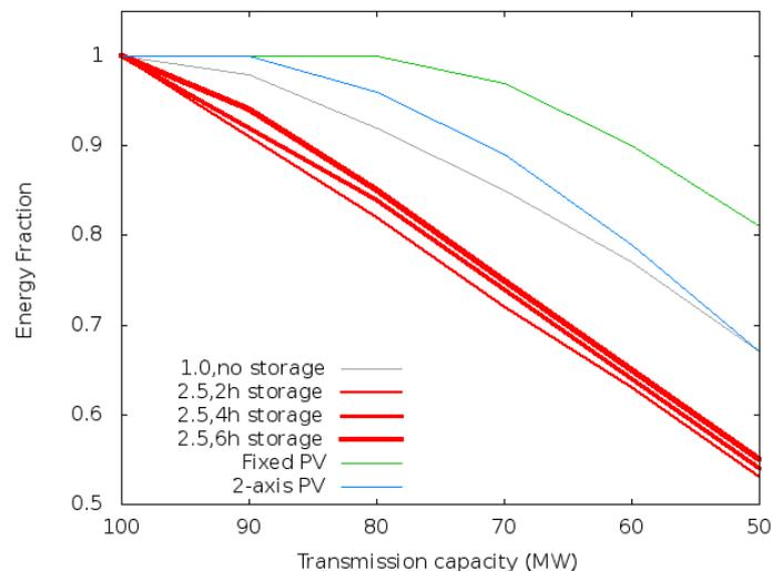
Figure 3: Energy production due to constrained transmission on CST and PV systems
