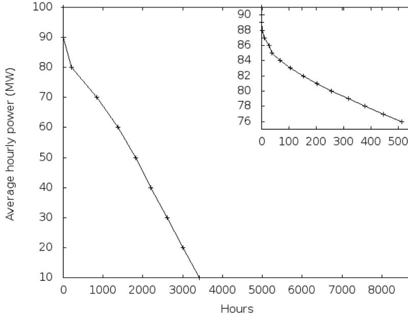
Figure 2: Power duration curve for fixed Cobar PV system in 2009
