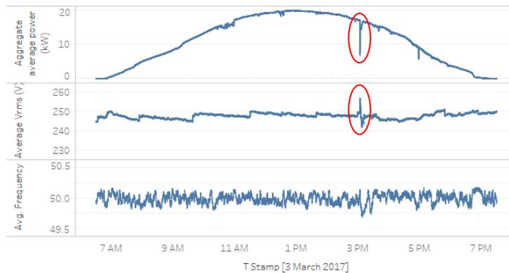
**Figure 3 Aggregate solar PV response to event (top), average local voltage (middle), average local frequency (bottom)**
